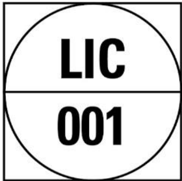
Part of a shared display and shared control in a DCS
